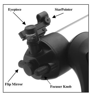
Attach the included accessories (eyepiece and Star Pointer finderscope) and remove the front lens cover. Turn-on the Star Pointer by rotating the dial on the side. (For instructions on aligning the Star Pointer see the *Assembly* section of the manual).
